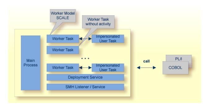
The CICS RPC Server can be configured to execute the RPC request impersonated under the RPC client user ID. For this, worker tasks start additional impersonated user tasks. This can be useful, for example for accounting. Impersonation is controlled by the ERXMAIN macro parameter IMPS.
