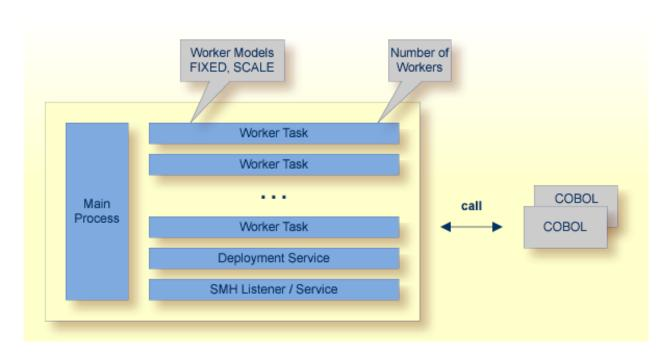
RPC requests are worked off inside the RPC server in worker tasks, which are controlled by a main task. Every RPC request occupies during its processing a worker task. If you are using RPC conversations, each RPC conversation requires its own task during the lifetime of the conversation. The CICS RPC Server provides two worker models:
