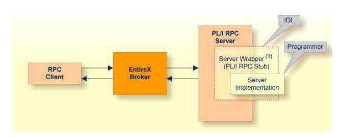
(1) The server wrapper is required for target platform IMS.
