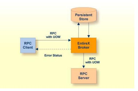
Reliable RPC is used to send messages to a persisted Broker service. The messages are described by an IDL program that contains only IN parameters. The client interface object and the server interface object are generated from this IDL file, using the EntireX C Wrapper.
