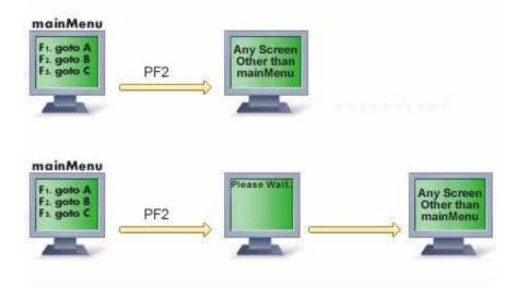
This example enables creating a Wait condition that pauses the procedure as long as the current screen is still "mainMenu" or as long as the "Please wait" message appears at the top of the screen. In addition it also prevents the procedure from hanging in an infinite loop from iterating more than 20 times. To accomplish this, a "Loop While" node with a complex condition, placing a Sleep Node inside the loop, should be used.
