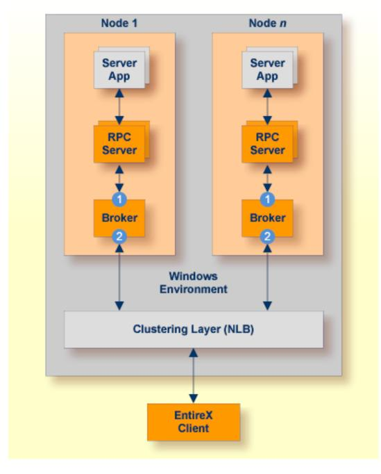
Segmenting dynamic workload from static server and management topology is critically important. Using broker TCP/IP-specific attributes, define two separate connection points:
