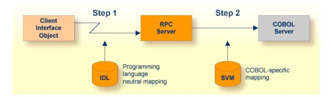
The RPC server marshalls the data in a two-step process: the RPC request coming from the RPC client (Step 1) is completed with COBOL-specific mapping information taken from the SVM file (Step 2). In this way the COBOL server can be called as expected.
