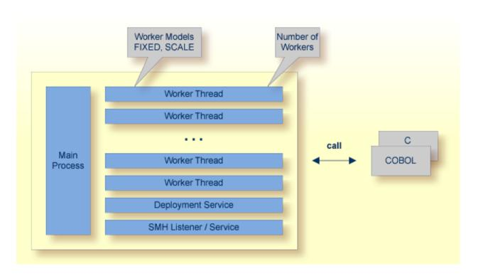
RPC requests are worked off inside the RPC server in worker threads, which are controlled by a main thread. Every RPC request occupies during its processing a worker thread. If you are using RPC conversations, each RPC conversation requires its own thread during the lifetime of the conversation. The BS2000/OSD Batch RPC Server provides two worker models:
