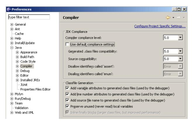
Click **Apply** to activate the settings. Eclipse will ask you to confirm the change, indicating that an internal rebuild is required. Reply **Yes**. The rebuild takes only a few seconds.
