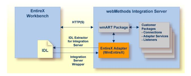
With the Integration Server Wrapper you can generate a server of type "RPC Listener" or "Reliable RPC Listener". See *Using the Integration Server Wrapper*.
