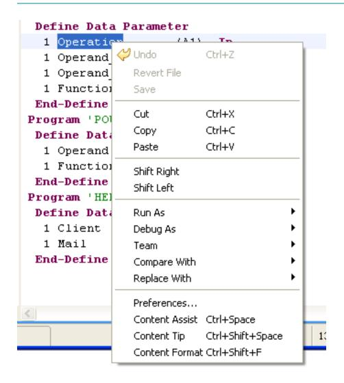
In addition to standard editor commands such as Undo, Revert File, Cut, Copy, Paste, Save etc., the context menu of the IDL Editor view offers two additional commands for shifting an element in the text: Shift Right to add a tab, and Shift Left to remove a tab.
