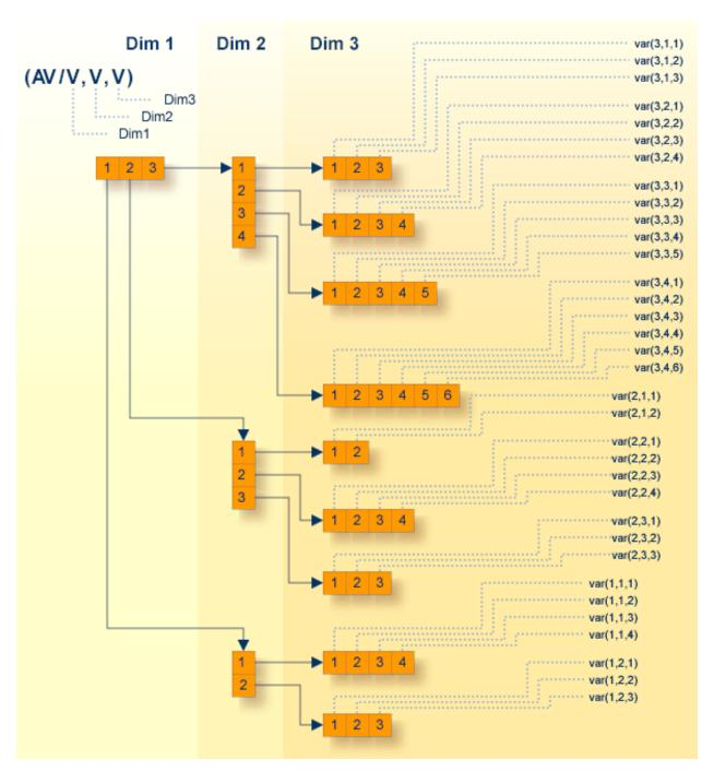
In the illustration above, the vectors of the second dimension have different lengths. The first vector has a length of 4, the second a length of 3 and the third a length of 2. The same is true for the third dimension with vector length of (3,4,5,6) (2,4,3) and (4,3).
