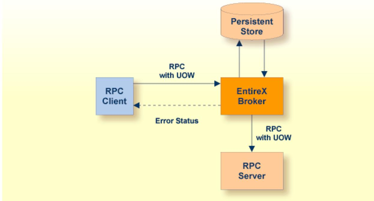
Reliable RPC is used to send messages to a persisted Broker service. The messages are described by an IDL program that contains only `IN` parameters. The client interface object and the server interface object are generated from this IDL file, using the EntireX DCOM Wrapper.
