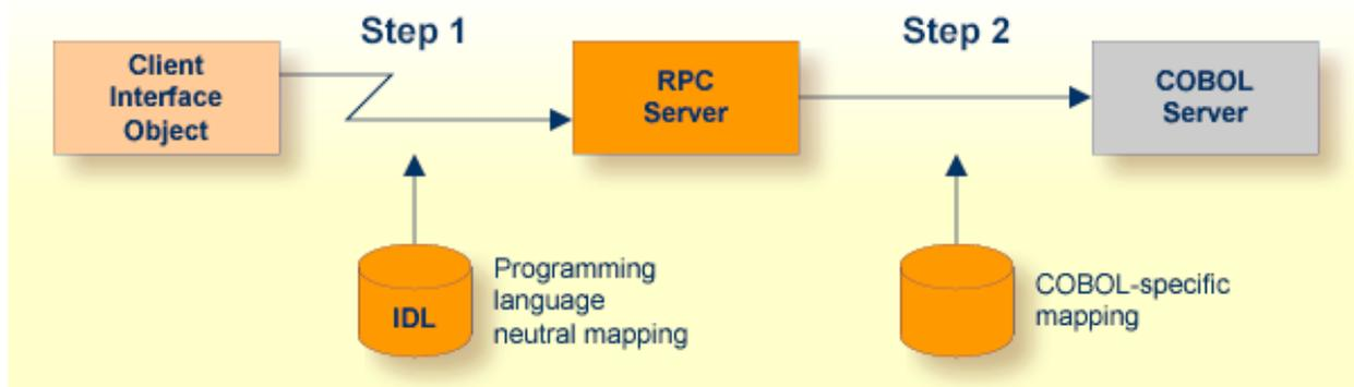
The RPC server marshals the data in a two-step process: the RPC request coming from the RPC client (Step 1) is completed with COBOL-specific mapping information taken from the server mapping file (Step 2). In this way the COBOL server can be called as expected.
