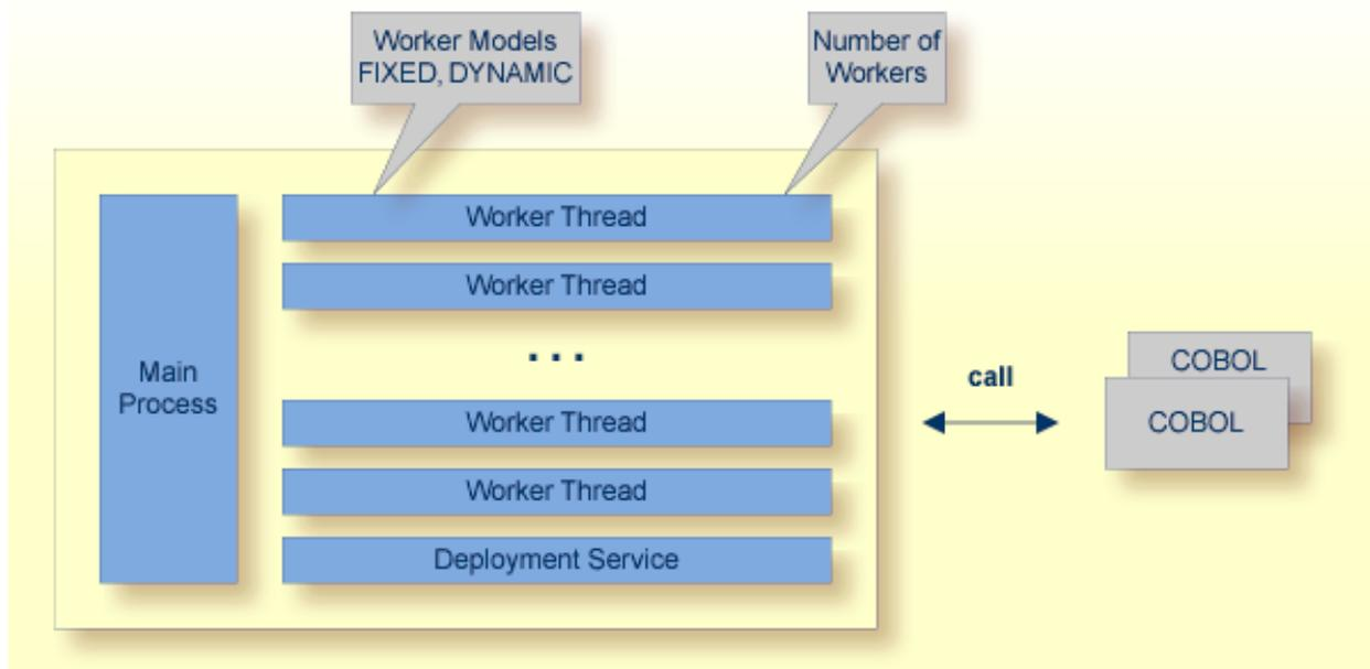
RPC requests are worked off inside the RPC server in worker threads, which are controlled by a main thread. Every RPC request occupies during its processing a worker thread. If you are using RPC conversations, each RPC conversation requires its own thread during the lifetime of the conversation. The RPC Server for Batch provides two worker models:
