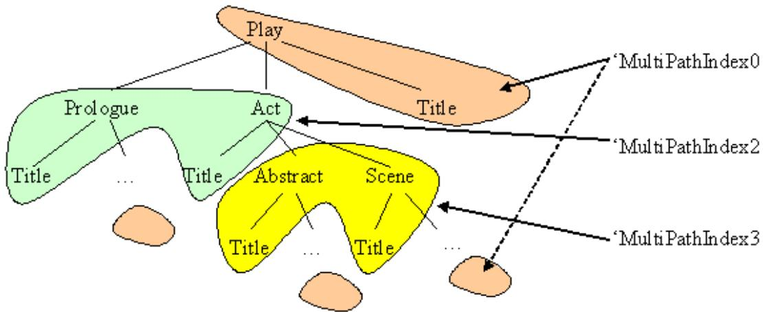
The picture shows which of these three indexes works with which parts of the structure tree. In TSD, the index definition looks like this:
