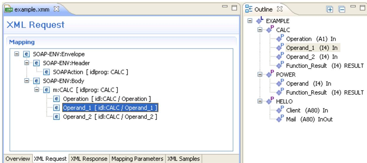
The XML Request shows the XML tree loaded or created so far for the selected IDL program. The XML tree can be modified in various ways. See [IDL to XML Mapping with the XML Mapping Editor](#).
