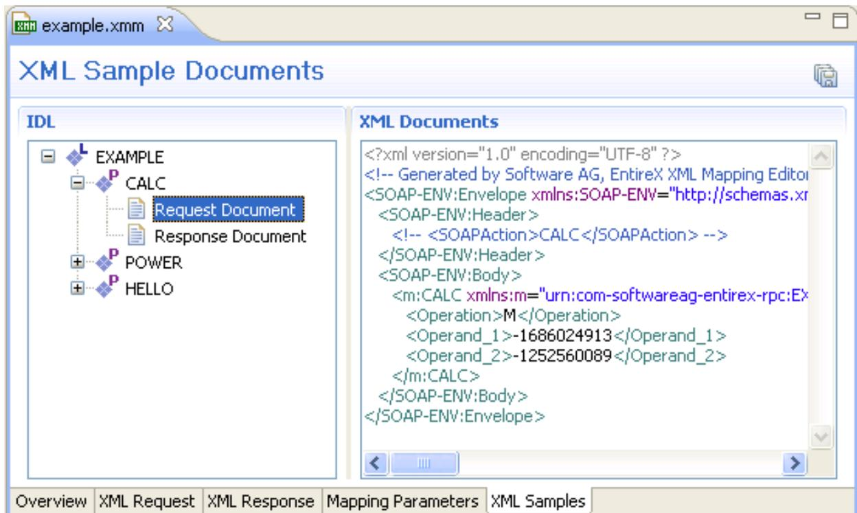
All generated XML Sample Documents can be stored in parallel to the selected XMM file by using the Save All toolbar button in the upper right corner of this page or the Save command in the context menu. The generated file name is built as follows:
