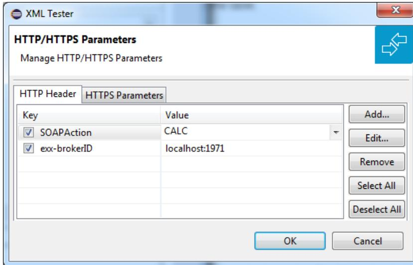
With the **HTTPS Parameters** tab you can set parameters required for an HTTPS connection. An entry must be selected to be active. The **Value** box holds the last five used values for the corresponding property. It is editable, which means you can change a value by clicking directly in the table.
