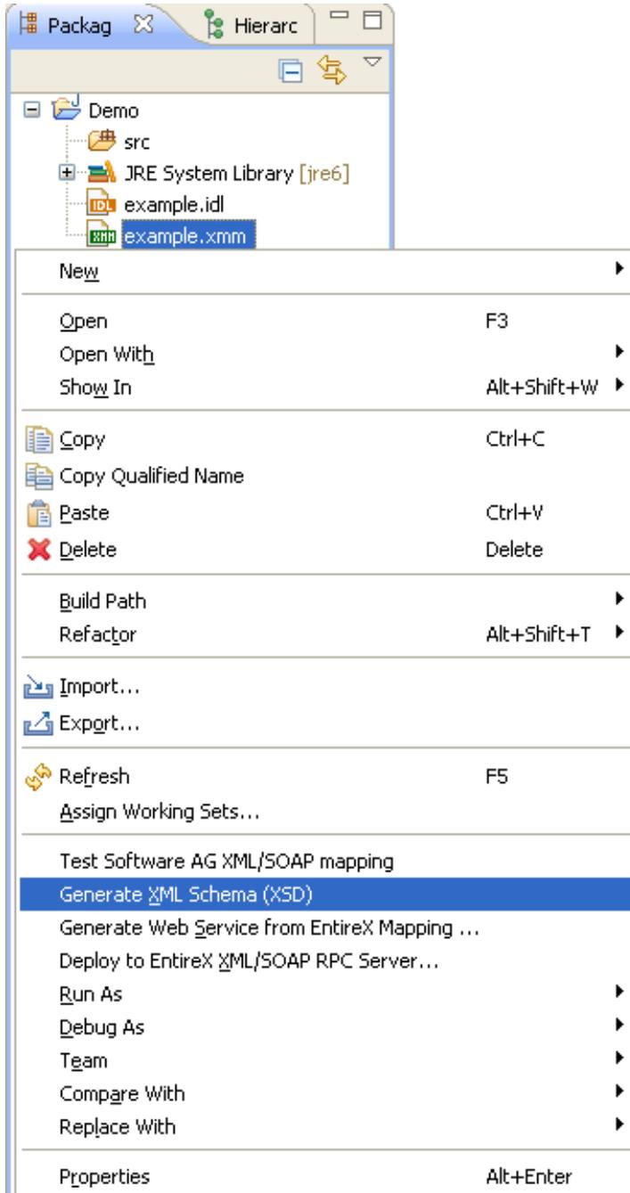
The generated XML Schema files will be stored in parallel to the selected XMM file, where one file represents the direction (request or response) and the defined prefixed element.
