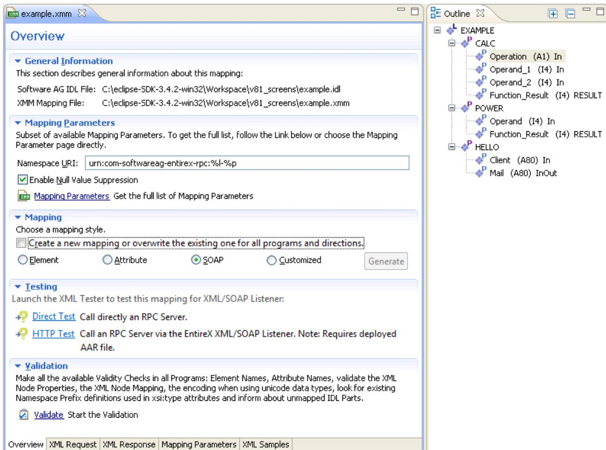
If no XMM file exists for the IDL file, the check box **Create a new mapping or overwrite the existing one for all programs and directions** is checked the mapping style is set to "SOAP" as default value. Choose the required mapping style and press **Generate**.
