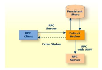
Reliable RPC is used to send messages to a persisted Broker service. The messages are described by an IDL program that contains only IN parameters. The client interface object and the server interface object are generated from this IDL file, using the respective Software AG component.
