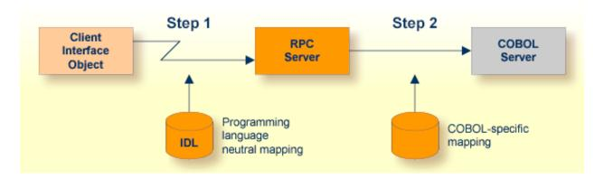
The RPC server marshals the data in a two-step process: the RPC request coming from the RPC client (Step 1) is completed with COBOL-specific mapping information taken from the server mapping file (Step 2). In this way the COBOL server can be called as expected.
