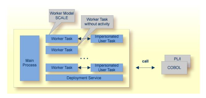
The RPC Server for CICS can be configured to execute the RPC request impersonated under the RPC client user ID. For this, worker tasks start additional impersonated user tasks. This can be useful, for example for accounting. Impersonation is controlled by the ERXMAIN macro parameter IMPS.
