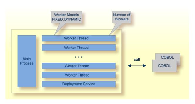
RPC requests are worked off inside the RPC server in worker threads, which are controlled by a main thread. Every RPC request occupies during its processing a worker thread. If you are using RPC conversations, each RPC conversation requires its own thread during the lifetime of the conversation. The RPC server provides two worker models:
