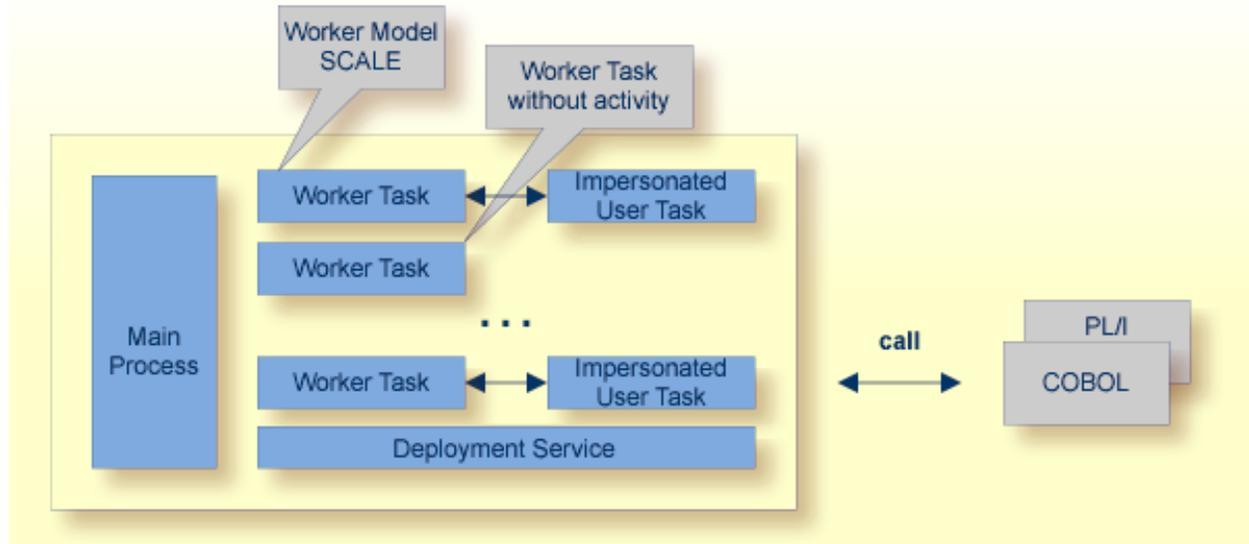
The RPC Server for CICS can be configured to execute the RPC request impersonated under the RPC client user ID. For this, worker tasks start additional impersonated user tasks. This can be useful, for example for accounting. Impersonation is controlled by the **ERXMAIN macro** parameter **IMPS**.
