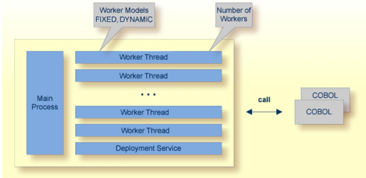
RPC requests are worked off inside the RPC server in worker threads, which are controlled by a main thread. Every RPC request occupies during its processing a worker thread. If you are using RPC conversations, each RPC conversation requires its own thread during the lifetime of the conversation. The RPC server provides two worker models:
