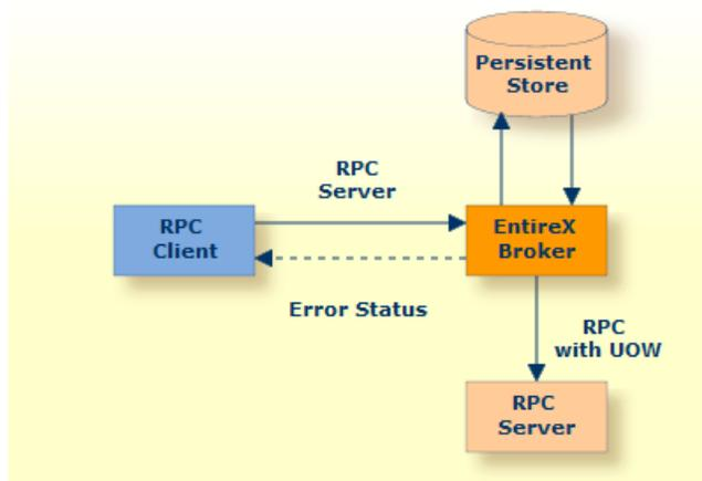
Reliable RPC is used to send messages to a persisted Broker service. The messages are described by an IDL program that contains only IN parameters. The client interface object and the server interface object are generated from this IDL file, using the respective Software AG component.
