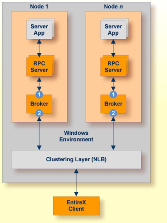
Segmenting dynamic workload from static server and management topology is critically important. Using broker TCP/IP-specific attributes, define two separate connection points:
