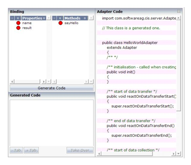
The properties and methods which cannot be found in the adapter code are indicated by red dots.
