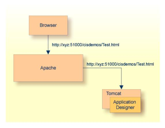
Apache is used as the web server to the outside world. All requests from outside are going through Apache. This means that only one server and one port is opened to the outside (typically the Apache server with port 80). Requests to Application Designer which runs, for example, on Tomcat under port 51000 are going as a "port 80" request to Apache and are routed from Apache as a "port 51000" request to the Tomcat server.
