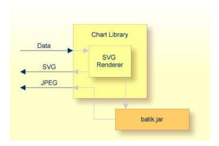
The library offers an API in which you pass the data to be rendered into a chart. It interprets the data and creates an SVG (scalable vector graphics) string out of it. This SVG string can be directly passed back to the calling application.
