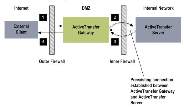
In an ActiveTransfer Gateway configuration, external clients send requests to ActiveTransfer Gateway (1). ActiveTransfer Gateway passes the requests to ActiveTransfer Server (2). After processing the requests, ActiveTransfer Server sends a
