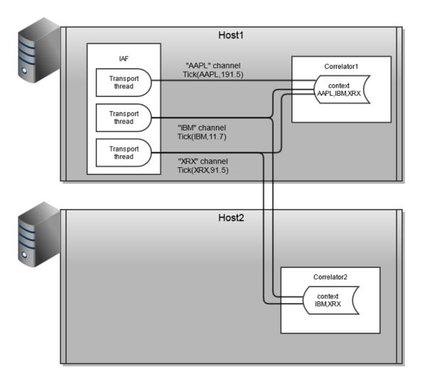
In summary, the partitioning strategy can be thought of as a formula for splitting and duplicating monitors and/or events between correlators while preserving the correct behavior of the application. In some circumstances, it may be necessary to re-write monitors that work correctly on a single correlator to allow them to be partitioned across correlators, as the following section describes.
