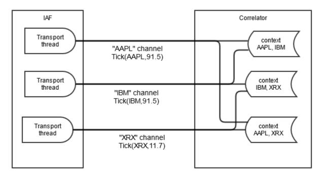
Again, each monitor instance is spawned to a new context and subscribes to the channels (stock symbols in this application) that it requires data for. Note that while the previous example would scale very well, this will not scale as well. In particular, if one monitor instance requires data from all or the majority of the channels, then it can become a bottleneck. However, there may be multiple such monitor instances running in parallel if they are running in separate contexts.
