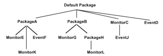
The root of the tree is the default package, which contains code that does not explicitly specify a package with the package statement. Specified packages are intermediate nodes. Packages can nest inside each other. Monitors and events in specified packages are leaf nodes. If you specify an event type in a monitor, that event is a leaf node and its containing monitor is an intermediate node.
