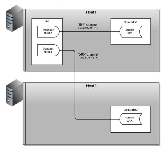
This configuration allows many contexts to run on two hosts and requires use of engine\_connect to set up the topology.
