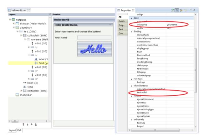
If a value for the testtoolid property is not explicitly set in a FIELD control, the HTML will contain a data-testtoolid attribute with the value of the valueprop property. This is shown in the HTML snippet below. You do not need to understand all the HTML details. The snippet just shows that a data-testtoolid attribute is automatically generated for a FIELD control; you do not have to do anything.
