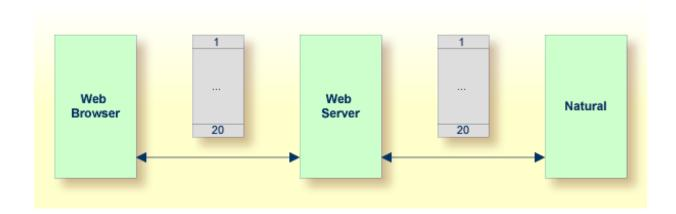
Step 2: When you scroll up and down, no server round trips to the web server or to the Natural application are performed.
