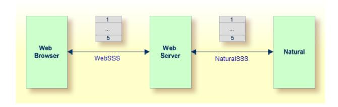
The Natural application can dynamically decide at runtime which option of server-side scrolling and sorting it wants to use. This can depend on the number of records contained in a search result.
