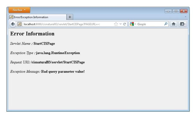
As an alternative to this default error handling servlet, you can add your own error handling servlets and/or error pages.
