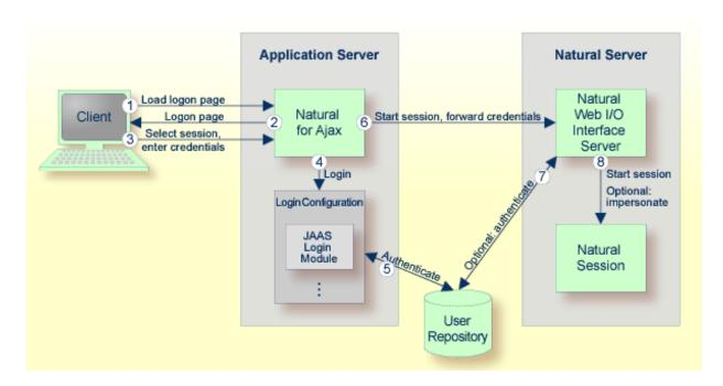
When application-managed authentication has been activated, the user is first authenticated on the application server or web container. For the authentication, JAAS-based (Java Authentication and Authorization Service) login modules are used. The login modules to be used and their parameters are configured in a login configuration. The user credentials entered on the Natural for Ajax logon page are authenticated against a user repository that is defined by the configured login modules.
