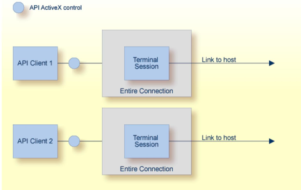
When a terminal session is in API mode, it is usually hidden to prevent user input. If the API makes the terminal visible, the user has full control of the terminal, including executing procedure files and closing down the terminal session. All data transfer operations and procedure files will still remain under the control of the API client.
