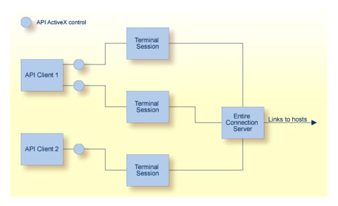
Each API control can link to an existing terminal session or create a new terminal session. Each terminal session can have one API control attached at any one time, the only exception being a terminal running in unattended mode when attaching is not allowed. It is also impossible to set an API-controlled terminal to unattended mode.
