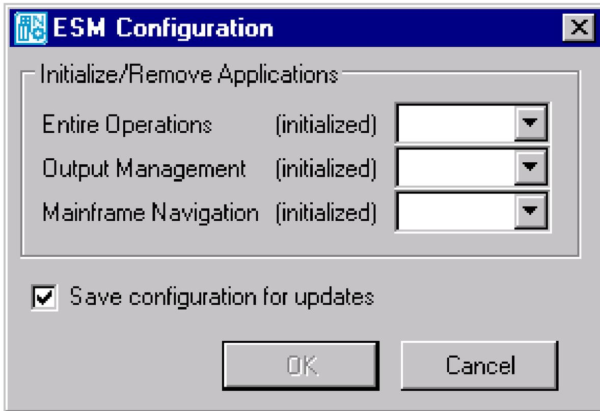
The ESM Configuration utility initializes or removes Entire System Management GUI components (applications) at your installation site.
