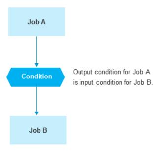
A specified event occurred as a result of Job A. This sets the condition, signaling to Entire Operations that Job B can be started.
