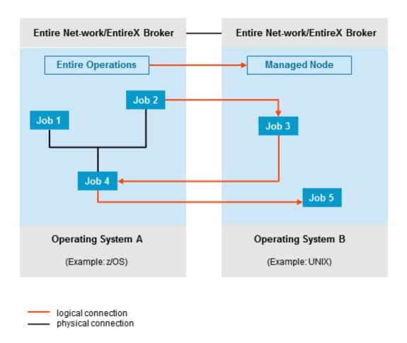
While the Entire Operations Monitor program handles the distribution and decentralized execution of processing steps, this type of distributed processing can still be monitored and controlled centrally from a single point of management.
