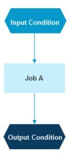
All input conditions must be fulfilled before a job can be submitted (prerequisite condition). You can define any number of input conditions for a job.
