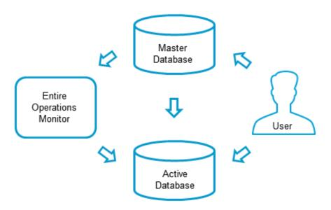
The master and active databases are located within the same physical database file.
