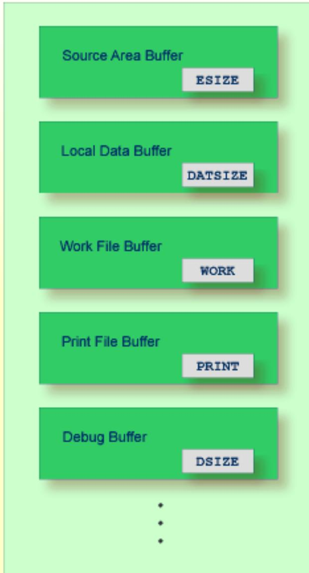
As illustrated in the diagram above, the size of a buffer can be specified with a Natural parameter, except for internal or variable Natural buffers. For example, the Natural profile parameter `ESIZE` determines the size of the source area assigned to a Natural editor for editing source code. The profile parameter `DATSIZE` determines the size assigned for holding local data from a Natural program (and subordinate objects if invoked by the program) at execution time.
