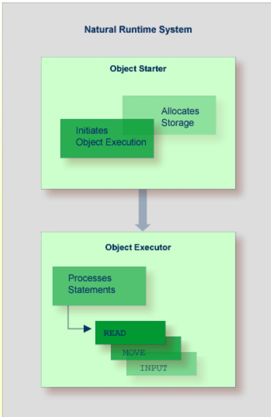
The Natural runtime system consists of two major components: the object starter and the object executor.
