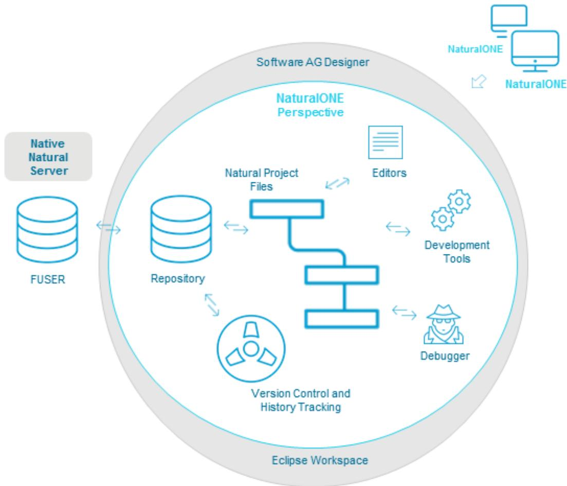
In NaturalONE, Natural applications are organized in projects. All Natural objects and libraries referenced by an application are contained in project files. The projects are contained in an Eclipse workspace that acts as an interface between the different tools provided for developing applications.
