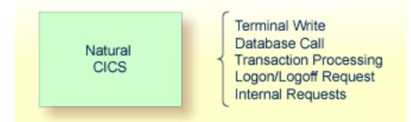
The figure above shows significant monitoring points between Natural and Natural Monitor. The Natural Monitor user interface allows the user to display data from these various monitoring points to evaluate performance and fine tune the system.
