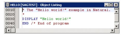
The window title shows the name of the object (here: HELLO) and the name of the library (here: SAGTEST) where the object is stored. The **Object Listing** window is identical to the window that appears when using the LIST system command.
