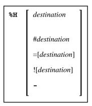
These terminal commands are used to produce hardcopy output from Natural reports on a printer or special destination, such as the source area.
