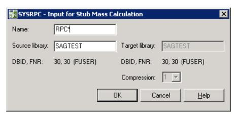
2. In the **Name** text box, enter the name of the subprogram for which to calculate the size or specify a range of names. The text box is preset to an asterisk (\*) for all subprograms. For valid names, see *Name* in *Specification and Compression*.
