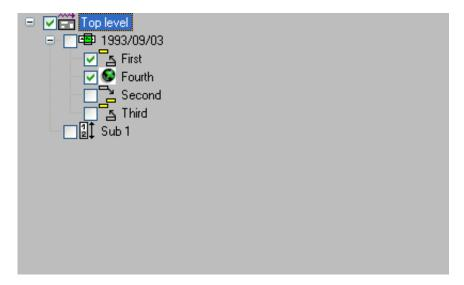
The tree view control shown above is specified with the "+/- buttons (b)", "Lines (l)", "Lines at root (r)" and "Check boxes (c)" STYLE flags.
