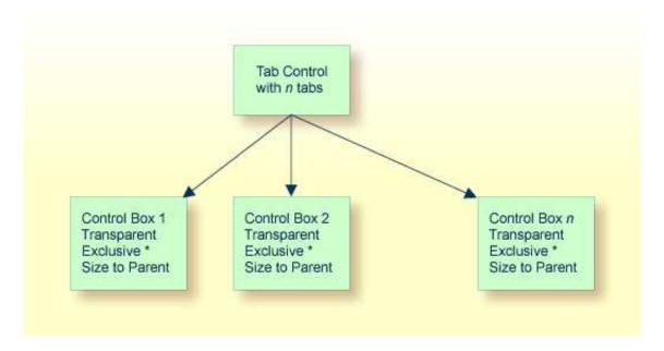
As shown in the diagram, each child control box should be transparent, that the tab control's background texture (if any) shows through, and have the "size to parent (z)" STYLE, so that the control boxes automatically exactly fill the interior area of the tab control, both immediately and whenever the size of the tab control is changed. In addition, each control box should be "exclusive" if the tab control is not UI active, such that only one child control box is visible at any time.
