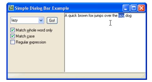
Setting the "dockable" state in the Dialog Bar Attributes window in the dialog editor causes the window to be draggable by the user. Note also that the dialog bar no longer extends to occupy the full length of the side to which it is docked (another dialog bar control or tool bar control could be docked underneath it):
