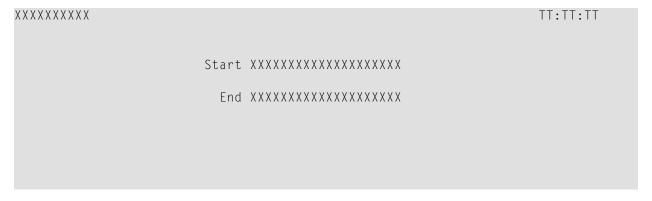
The first line of the map contains system variables for the current date and time. There are two data fields (input fields) in which the user can specify a starting name and an ending name. The data fields are preceded by text fields (labels).
