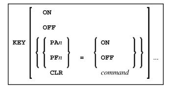
This command is used to assign functions to keys on the keyboard of video terminals. Moreover, you can change, activate and deactivate the assigned functions.
