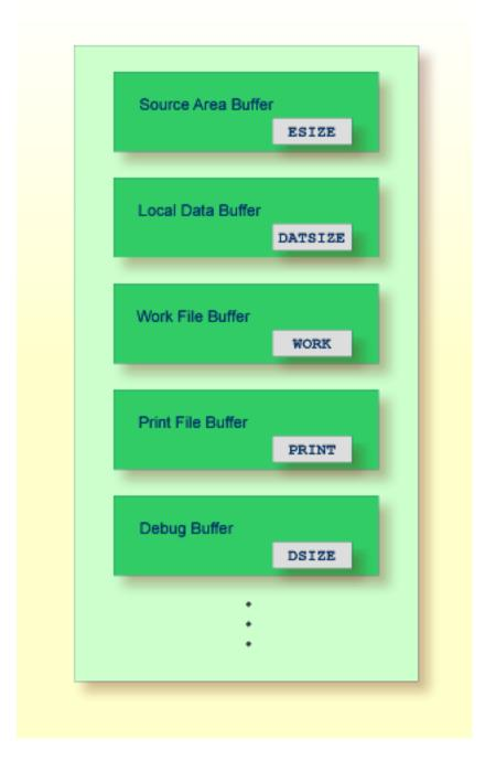
As illustrated in the diagram above, the size of a buffer can be specified with a Natural parameter, except for internal or variable Natural buffers. For example, the Natural profile parameter ESIZE determines the size of the source area assigned to a Natural editor for editing source code. The profile parameter DATSIZE determines the size assigned for holding local data from a Natural program (and subordinate objects if invoked by the program) at execution time.
