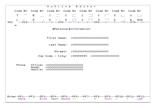
The upper part of the outline editor screen shows all valid box codes (for example, O), symbols for the type of box they create (for example, a square  $\Box$  for O) and the end marker E (END). This chart is not displayed in full-screen mode.
