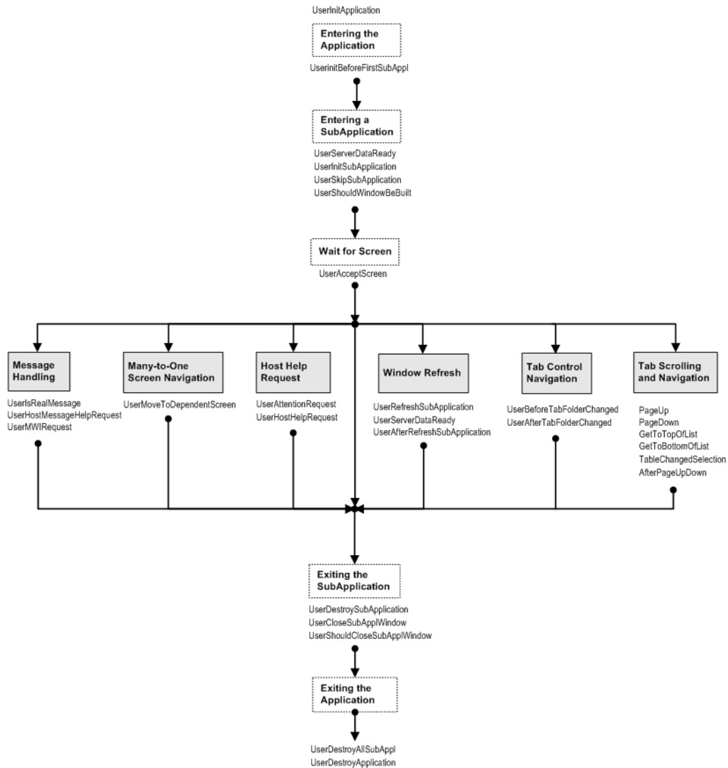
Figure 159. Flow of events and system-triggered methods
