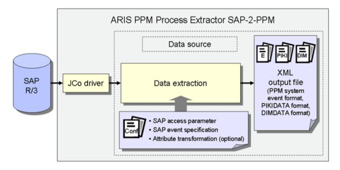
The SAP Java Connector (SAP JCo) is used to establish the connection to the SAP system using SAP access parameters. Data is then extracted from the SAP tables in accordance with the SAP event specification. Finally, an optional attribute transformation takes place and the data is output to XML files in a PPM-compatible output format.
