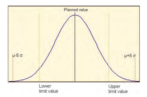
The aim of the Six Sigma method is for almost 100% (more precisely 99.99966%) of all results for a process to lie within a range that stretches from  $\mu$ -6 $\sigma$  to  $\mu$ +6 $\sigma$ . In other words, this means that out of a million executions only 3.4 results will have errors.
