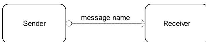
Figure 2: Implicit modeled message object (no message structure defined)
