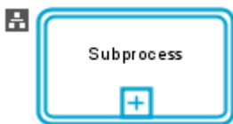
Figure 225: Symbol for a collapsed transaction
