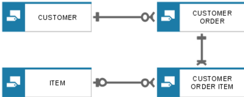
Figure 50: Data model in IE notation
