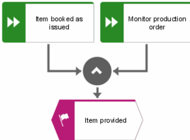
Figure 97: AND operator of functions with created events
