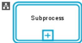
Illustration 165: Symbol for a collapsed transaction
