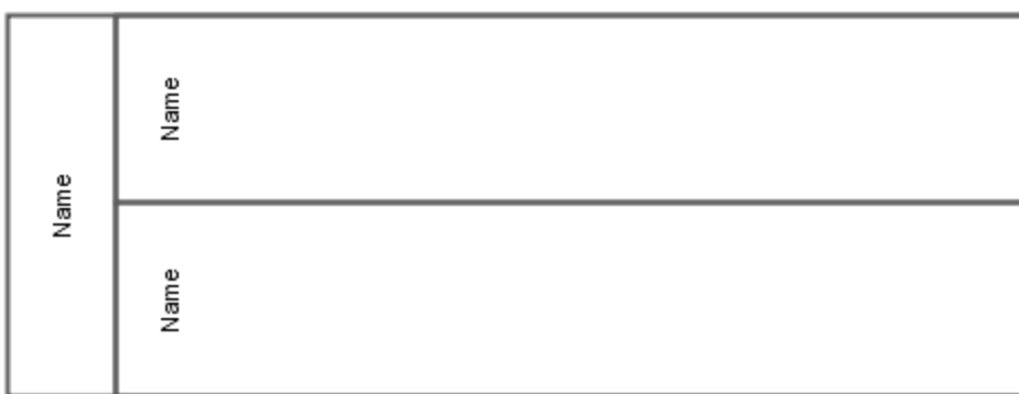
Figure 205: Pool with two lanes according to BPMN
