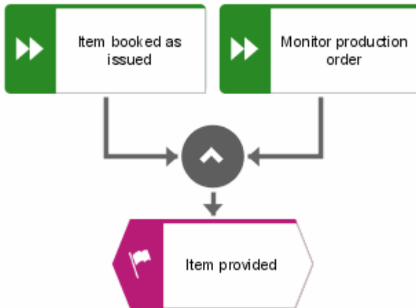
Figure 78: AND operator of functions with created events
